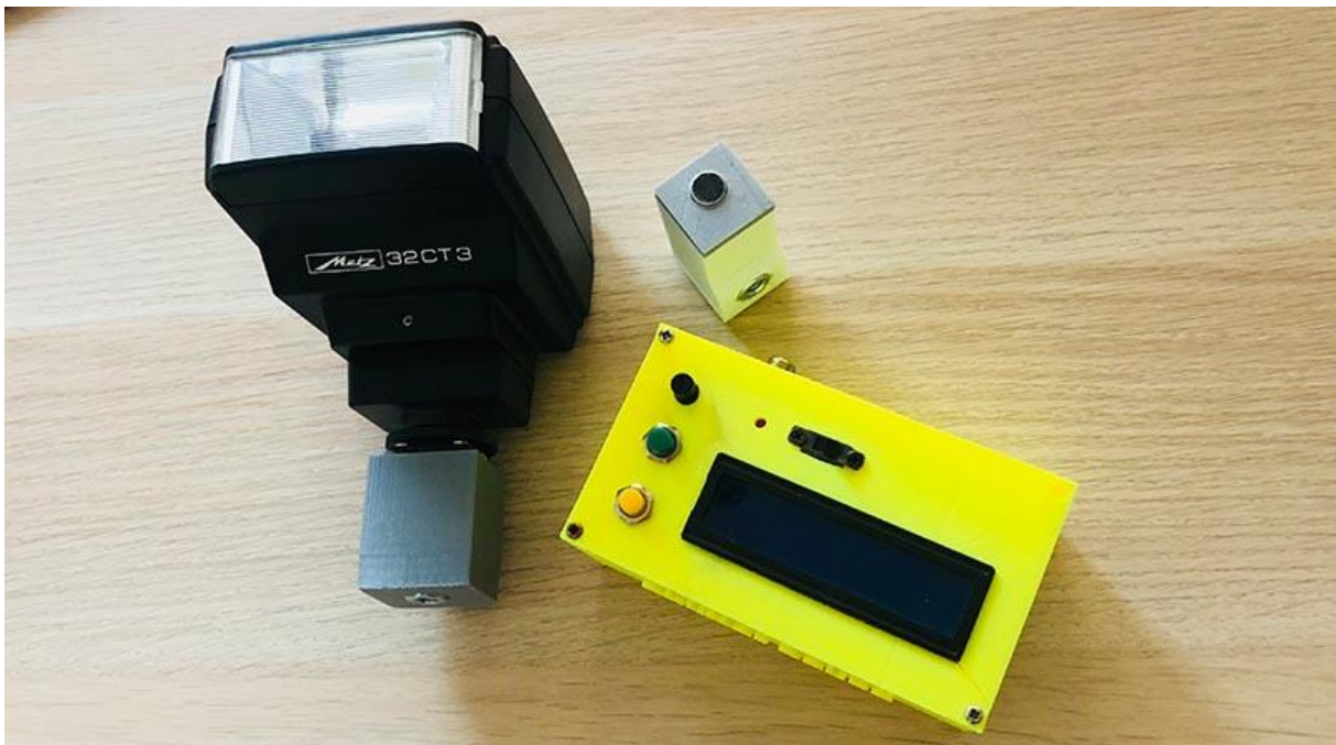
Fig. 2: All necessary components for the Shutter Sound project. The external flash is mounted on a flash shoe and equipped with a ¼ inch nut for a tripod. The other grey box includes the sound sensor. The yellow box includes the Arduino Nano.
